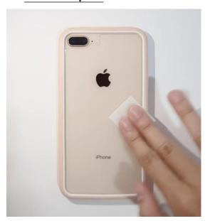
Align the center of the four metal pads and target the center of the device or phone case.
